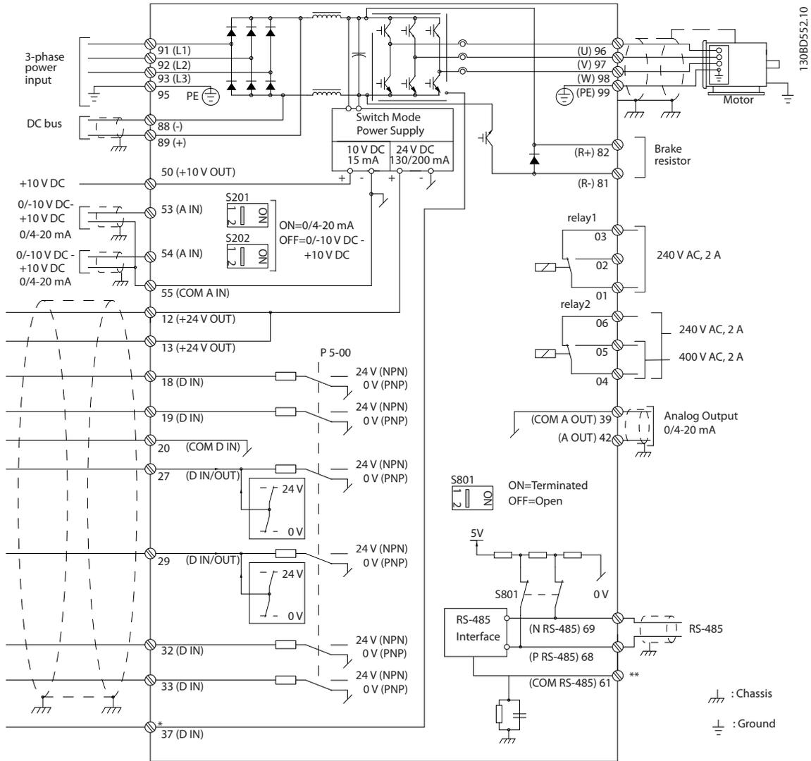
Illustration 4.1 Basic Wiring Schematic
